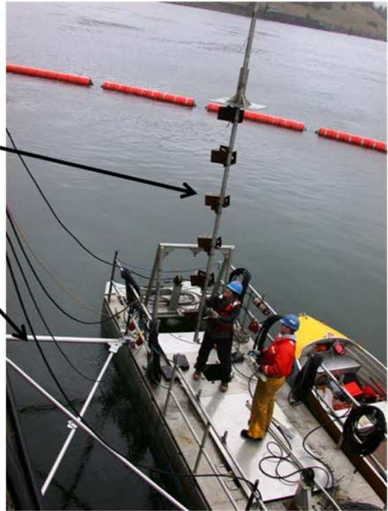
Figure 1. Equipment barge for monitoring B2CC passage using DIDSON cameras. Photos are from a study conducted in 2008.
